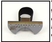
The Finger Jig alignment tool is used to hold double edge splice tapes (without onboard pin jigs) for quick and easy splicing of carrier tapes on-the-fly. It includes an elastic finger band, as well as a set of alignment pins mounted on the tool, and is used by the operator right at the placement machine. The jig is used to splice any tape width in the palm of your hand. It is used with either metal
