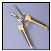
The 8mm tape cutting tool can be used with either paper or plastic tape, punched or formed pockets, and any cover tape. This model cuts 8mm wide tapes only and includes an alignment block with 2 sets of locating pins; one for 1mm pitch (8mm wide tape and 0201 and below pocket sizes) and one for 2mm pitch (8mm wide tape and 0402 and above pocket sizes).
