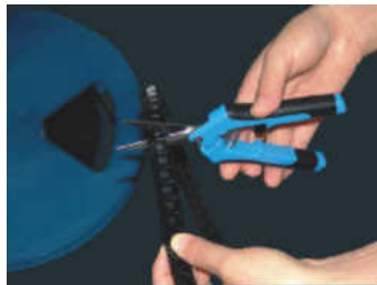
PIC 3: View of splice cutter for larger tape. Tape will be cut between pockets.
