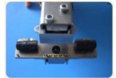
PIC 4: View of brass splice clip on locator pins of splice tool.
