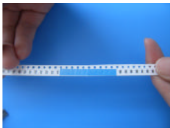
TOP VIEW Finished Splice
