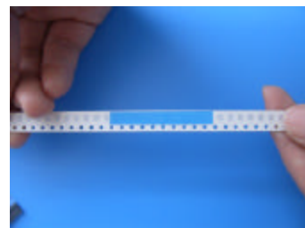
BOTTOM VIEW Finished Splice
